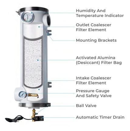
Super-Dry Compressed Air Dryers contains two highly efficient polypropylene coalescer elements at inlet & outlet ports to absorb oil and all solid air particles. Also included, one desiccant bag specifically designed to absorb water vapors and humidity from your compressed air system.
