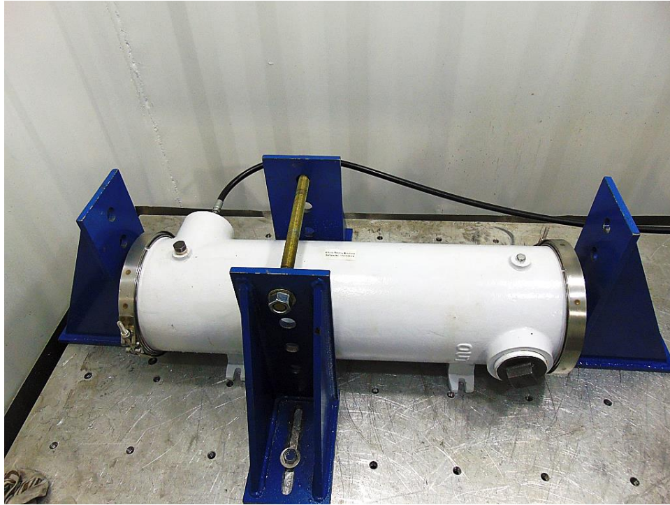
Figure 13: Sample 17010350-4 Trial #2 overall setup inside the pressure test chamber
