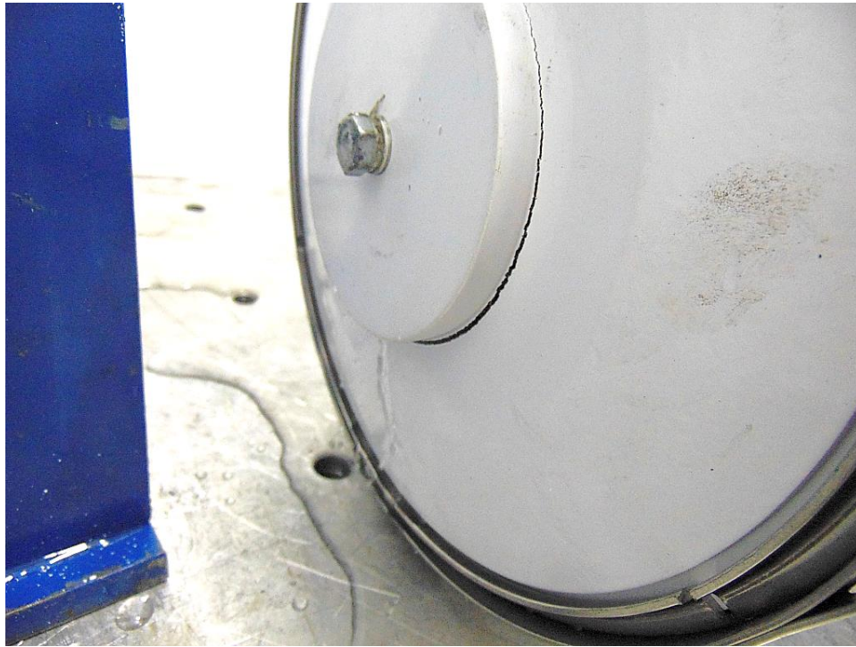
Figure 15: Sample 17010350-4 Trial #2 cracked at lid at 428 psi
