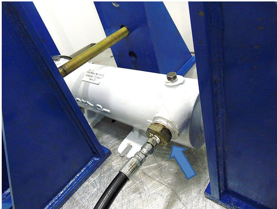
Figure 2: Sample 17010350-1 Trial #1 inlet connection
