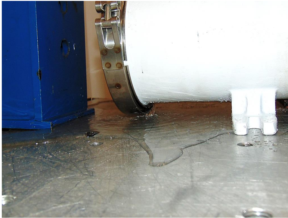
Figure 11: Sample 17010350-3 Trial #1 failed at lid/clamp at 650 psi
